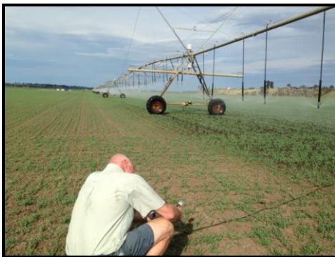
Checking end of LM residual pressure
