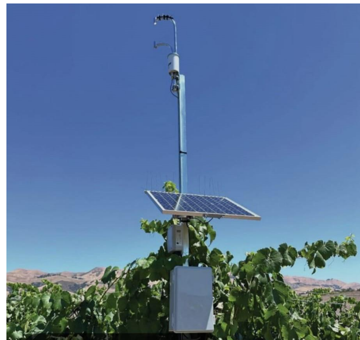
LI-710 Evapotranspiration Sensor - 9000-02 IoE Module, includes Base, Tower, and Solar Power
