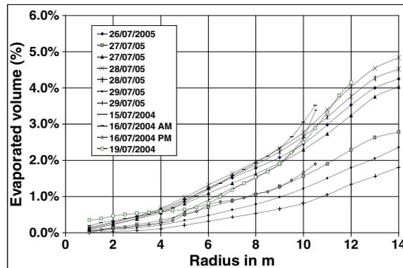
Figure 4. Per cent evaporation losses as a function of distance, tests performed outdoor in controlled conditions (no wind). This figure is available in colour online at [wileyonlinelibrary.com/journal/ird](http://wileyonlinelibrary.com/journal/ird)
