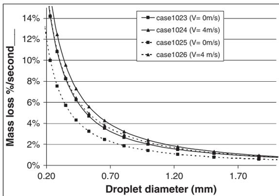
Figure 8. Effect of wind velocity on direct evaporation
