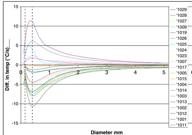
Figure 7. Difference in droplet temperature between injection and the end of flight as a function of droplet diameter. This figure is available in colour online at [wileyonlinelibrary.com/journal/ird](http://wileyonlinelibrary.com/journal/ird)
