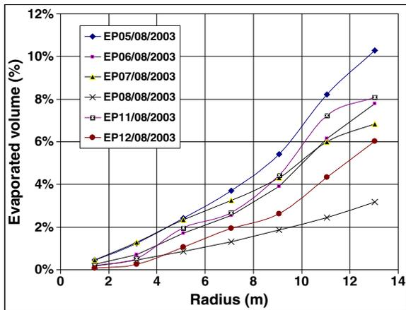
Figure 3. Per cent evaporation losses as a function of distance for field tests. This figure is available in colour online at [wileyonlinelibrary.com/journal/ird](http://wileyonlinelibrary.com/journal/ird)
