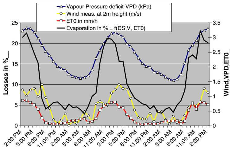
Figure 5. Simulation of evaporation losses on two summer days in 2005 in the south of France. This figure is available in colour online at [wileyonlinelibrary.com/journal/ird](http://wileyonlinelibrary.com/journal/ird)
