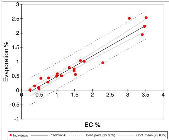
Figure 2. Evolution of electrical conductivity (EC%) of water samples during evaporation. This figure is available in colour online at [wileyonlinelibrary.com/journal/ird](http://wileyonlinelibrary.com/journal/ird)
