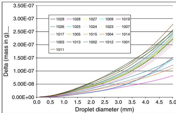
Figure 10. Evaporation losses of mass per unit time according to droplet size. This figure is available in colour online at [wileyonlinelibrary.com/journal/ird](http://wileyonlinelibrary.com/journal/ird)
