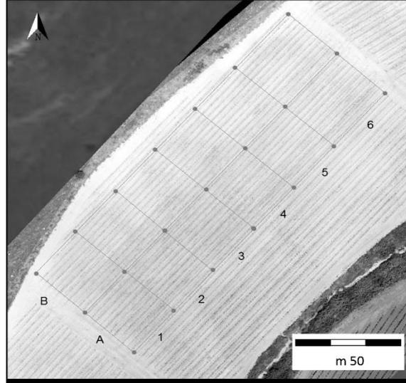
Figure 1. VRDI system layout; 2 strips, 6 zones each (A1-A6; B1-B6); each zone can be independently irrigated.
